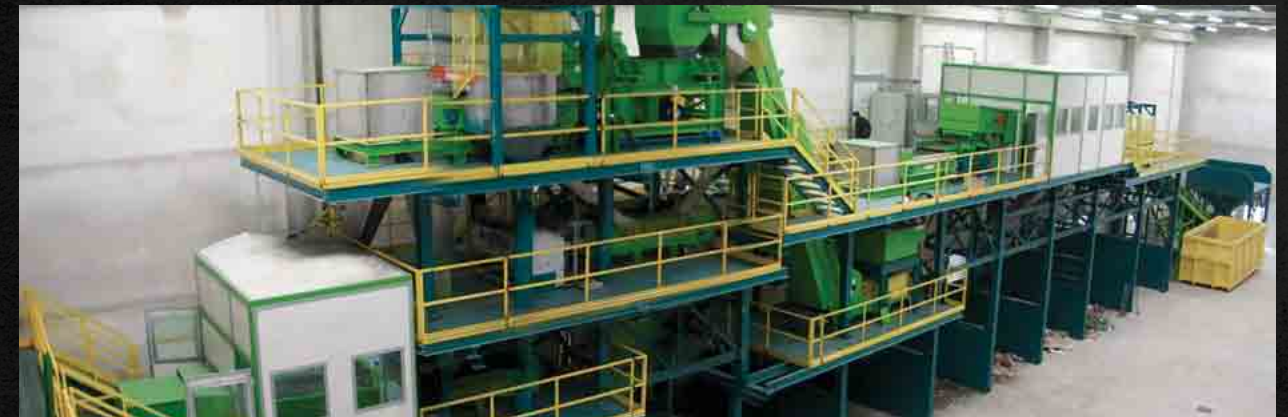
Glass recycling plant with Cogelme Eddy Current Separators, Magnetic separators and Glass crusher.
